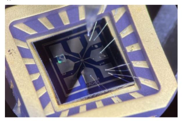
**Image 2.** An Archer 4 x 4 mm single-chip quantum electronic device after installing and bonding into a commercial chip carrier. This completed device is compatible with measurement setups for electronic characterisation at cryogenic temperatures as well as ambient conditions at room temperature using Archer's in-house lab capabilities as well as external facilities.
