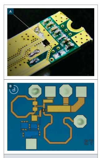
A - The integrated single chip ESR detector based on HEMT.
