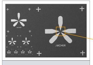
An example of typical electronic nanodevices fabricated towars qubit readout. The complex features, that appear as a lighter shade, are of various sizes and proximity, purpose developed for initial quantum measurements on cluster, few, and single qubits.
