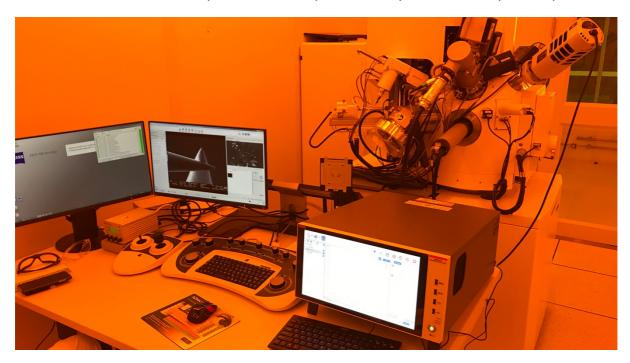
**Image 1.** Set-up of a measurement being performed on <sup>12</sup>CQ chip qubit components at the University Research and Prototype Foundry. The measurements require access and use of specialised instrumentation, like the ones pictured, to be performed successfully. The orange appearance is part of the sterile protocol inside the Research and Prototype Foundry.
