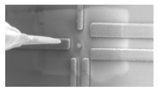
**Image 2.** A single qubit component undergoing direct quantum measurements related to the materials' electronic characteristics, with the qubit component observed in the centre of the image (round particle of about 50 nanometres in size) and surrounded by rectangular nanoelectrodes prepared using facilities at the University.
