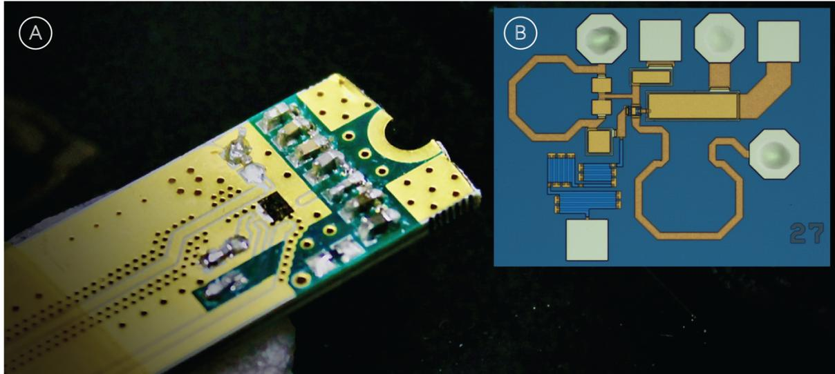
**Image 1. A** The integrated single chip ESR detector based on HEMT. **B** A microscope image of a region in **A** (inside the black square in the centre of the chip) of approximately 0.5mm x 0.5mm showing the miniaturised on-chip ESR componentry used to detect the quantum spin states in Archer's <sup>12</sup>CQ qubit material at room temperature.
