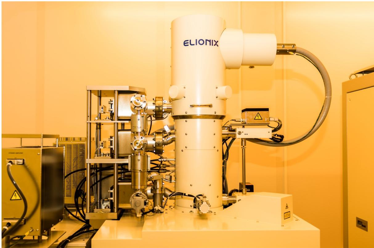
**Image 1. Elionix ELS-125 electron lithography system.** The vertical circular tower is where the electron-beam is located, while the chip is introduced through the load lock (the rectangular area with the protruding rod). The multi-million-dollar E-beam system is housed in a cleanroom environment in Sydney, Australia, and is manufactured in Japan.
