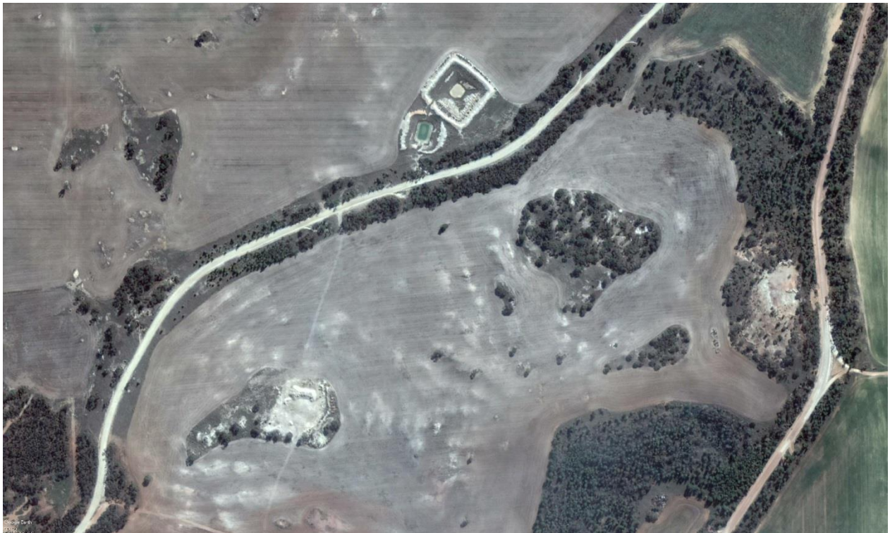
Fig. 2. Google Earth image showing outcropping kaolin (white colour) within the Kelly Tank Exploration Target area.
