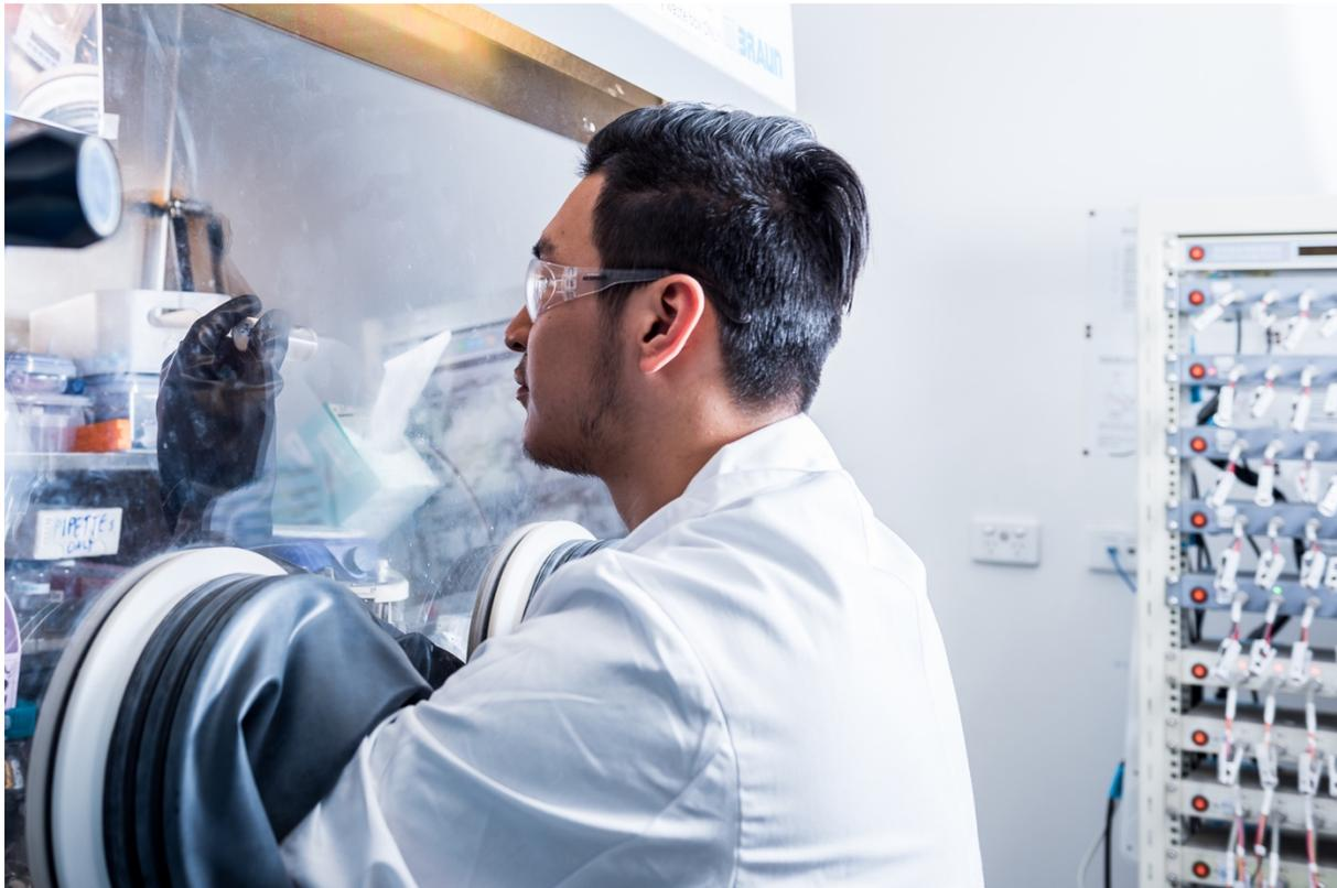
**Image 1.** Battery materials formulation, assembly and testing incorporating Archer Campoona graphite being performed at the University of New South Wales. Tightly controlled chemical and physical environments were used and required to handle battery componentry, with testing being conducted at small-scale levels.
