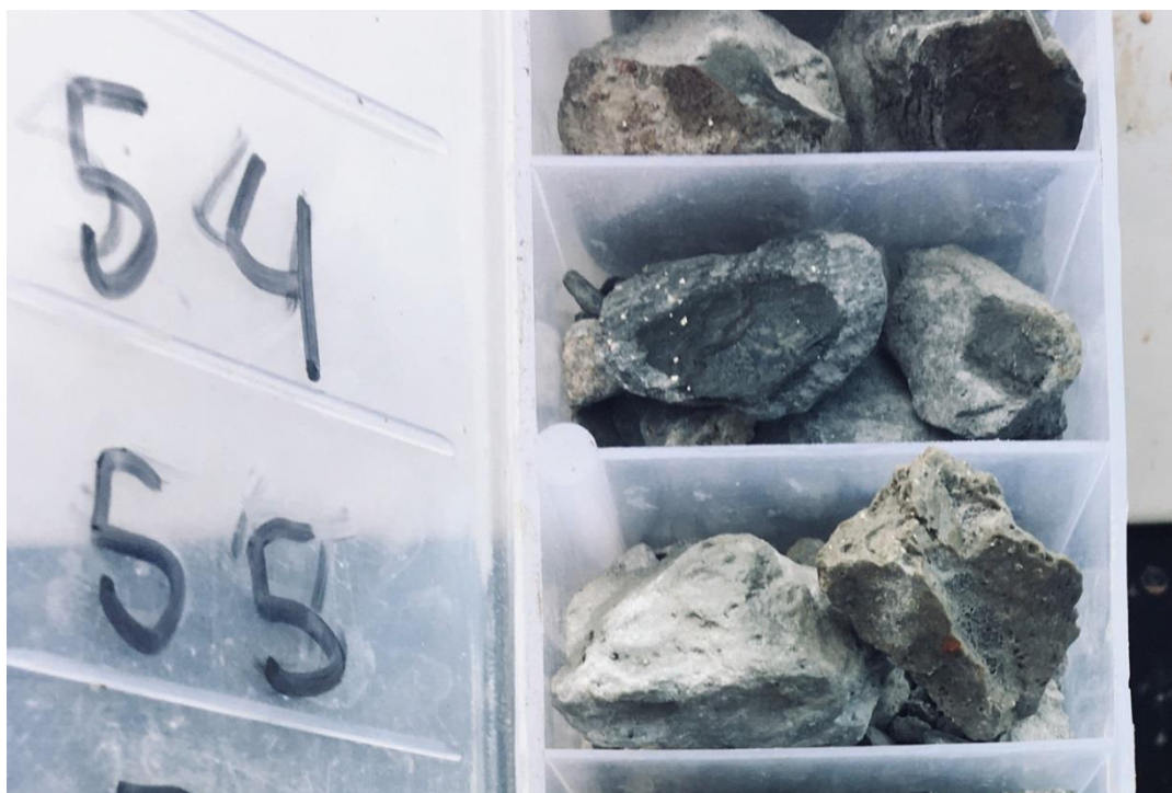
Plate 1. HDRC19-01 depths 54 and 55m showing the bleaching at 55m (sodic alteration).
