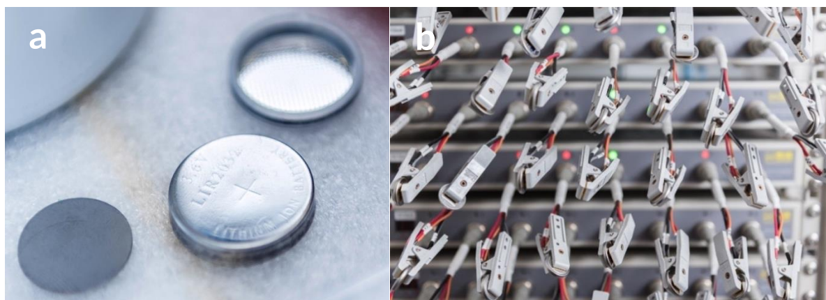
Fig. 2. a. Coin-cell battery assembly used for the full-cell configurations incorporating Archer Campoona graphite and the commercially relevant cathode chemistries. b. Coin-cell batteries assembled with full-cell configurations incorporating Archer Campoona graphite anodes and the commercially relevant cathode chemistries NMC, LFP, and LCO. The clips holding the coin-cells measure the charge and discharge properties of the battery to validate performance.
