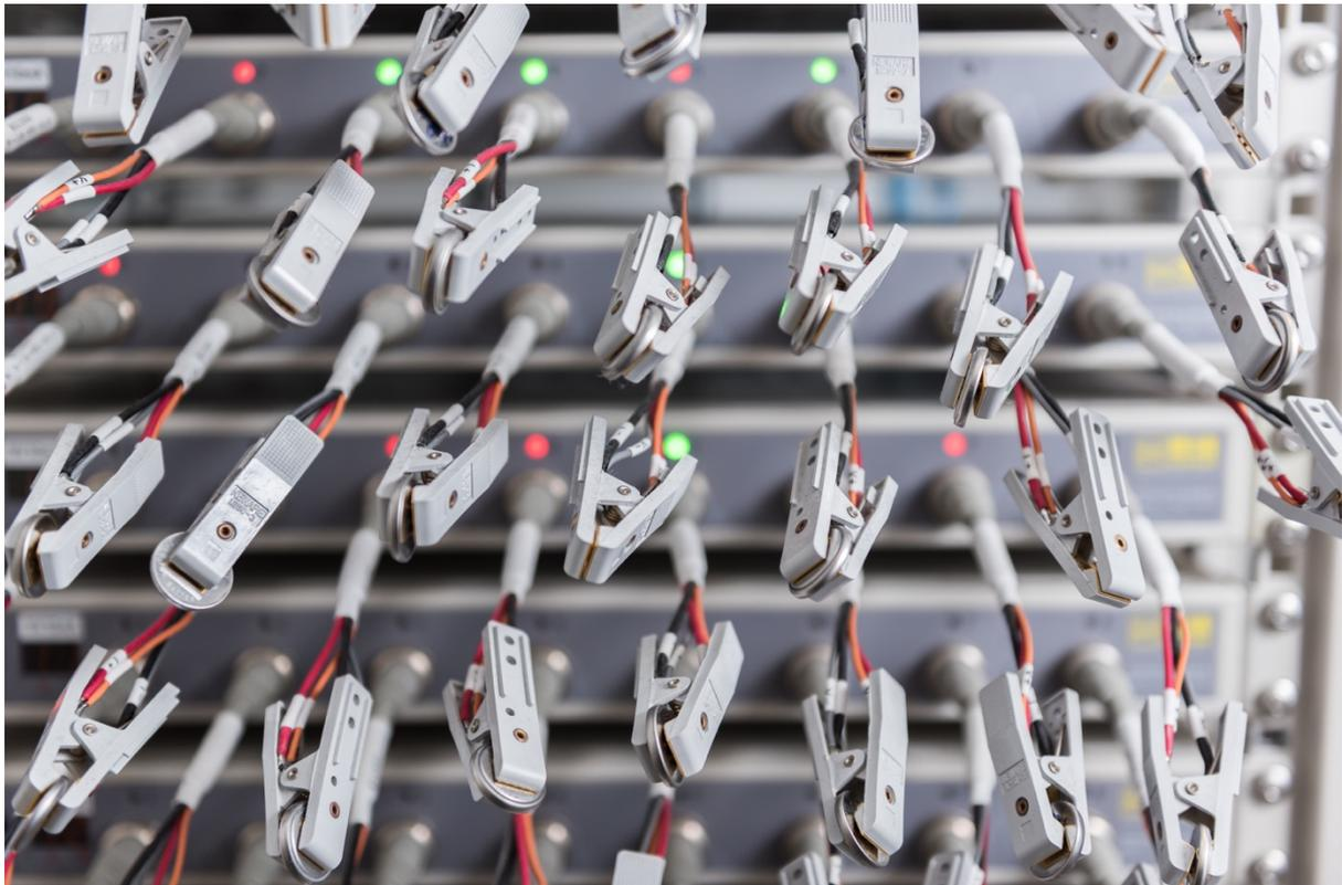
**Fig. 2.** Coin-cell batteries assembled with full-cell configurations incorporating Archer Campoona graphite anodes and the commercially relevant cathode chemistries NMC, LFP, and LCO. The clips holding the coin-cells measure the charge and discharge properties of the battery to validate performance.
