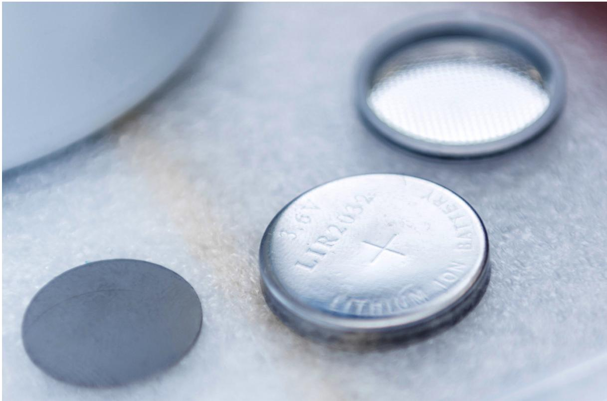
**Fig. 1.** Coin-cell battery assembly used for the full-cell configurations incorporating Archer Campoona graphite and the commercially relevant cathode chemistries.
