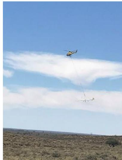
Figures 2 and 3: Geosolutions TDEM survey equipment at Blue Hills.
