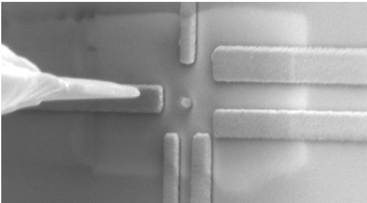
**Image 2.** A single qubit component undergoing direct quantum measurements related to the materials' electronic characteristics, with the qubit component observed in the centre of the image (round particle of about 50 nanometres in size) and surrounded by rectangular nanoelectrodes prepared using facilities at the University.
